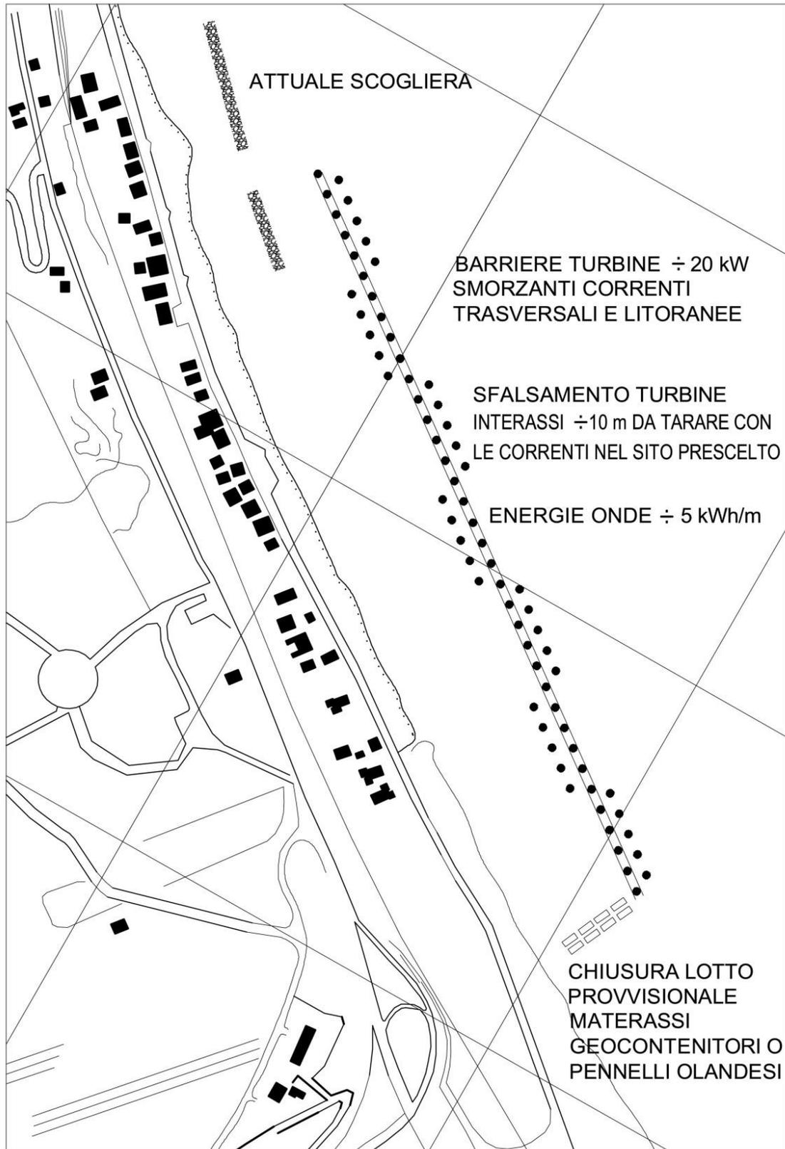
**Fig. 3 Turbines planimetry and distribution to be adapted at marine geomorfology in replacement of the nourishment and the cliffs**
