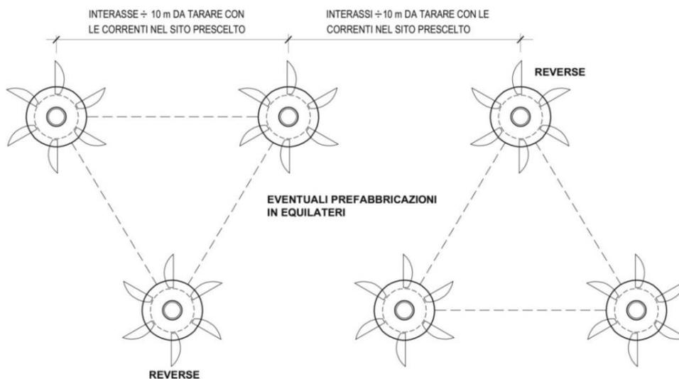
**Fig.2 Turbines supported on recycled plastic tubes in 3D printed, vibroinfixed in seabed at suitable depth through triangular prefabricated piles foundations.**
