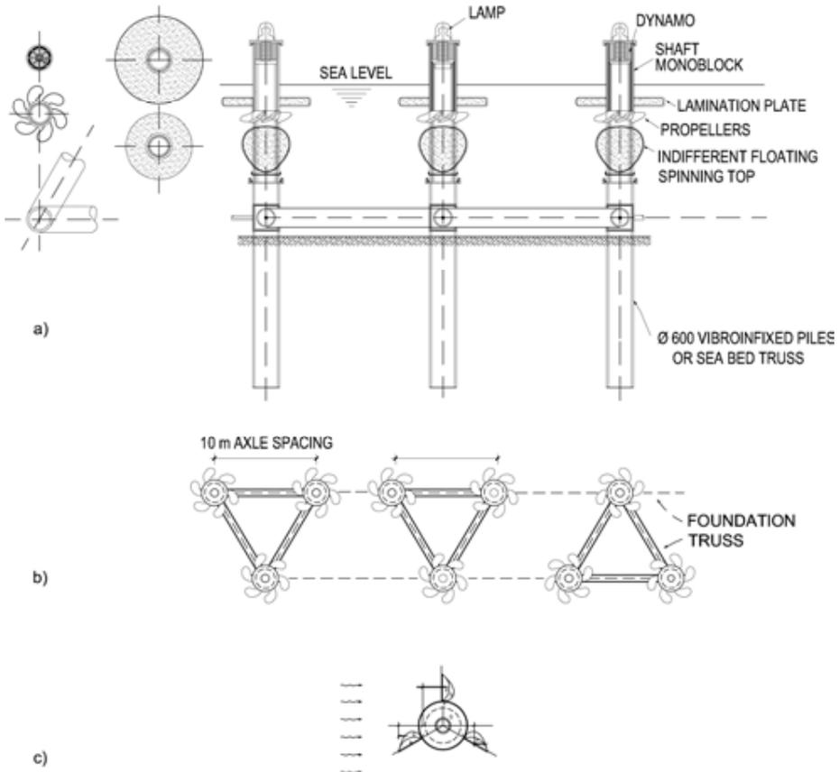
Figure 6 - a) Turbines with indifferent floating monoblocks (patent n° 0001411057; database CNR SOLAR code 9861TR2019) are pivoted on tubes. The pile-tubes are vibroinfixated in the sea bed, or founded on a reticular truss placed on the seabed, similar to a naval wreck; the whirligig is filled with sponge to prevent infiltrations from impacts; the propeller, whirligig and piles are printed in 3D using metal powder made from recycling machine scrap, or internal piles in fiber-reinforced.
